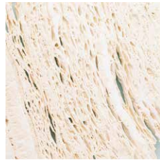
Travertino Travertino filled with epoxy resin
